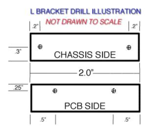
Stuff the new 440C cap PCB and install the Bracket with 4/32 harware. Loctite the nuts.
