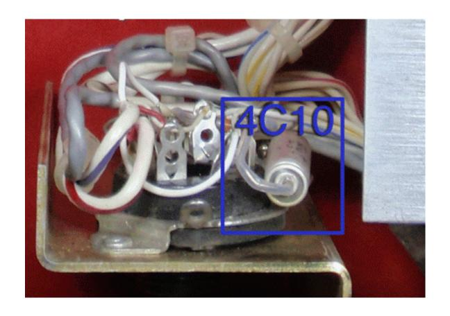
wire the new PCB starting with the 5 wh/red wires
