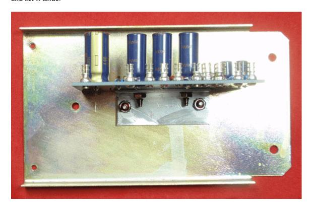
Cut the wires off the old caps at their terminals leaving the wires as long As possible. Strip and tin the wire ends. Set the old Mallorys aside complete With the 4 resistors and 1 diode. These will be replaced with new parts On the PCB.
