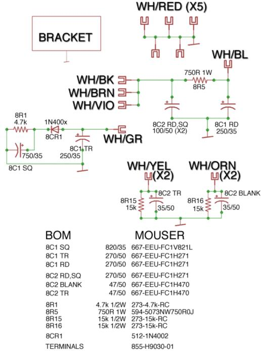
Note that the 750R 1Watt resistor replacement part is physically much smaller Than the old carbon comp 1 watt guy. The new guy really is 1 watt.
