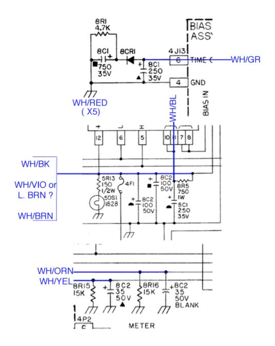
Note that 8C2 RD and 8C2 SQ are 2 100uf caps in parallel and will be replaced By one 270uf cap
