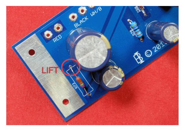
I would use an extra piece of wire to extend the ORN WIRES and and solder the other end to the lifted resistor end using heat shrink to insulate the connections.
