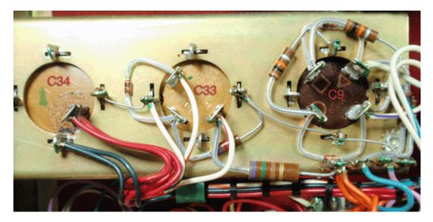
Note that the 750R resistor does not connect to C34 like the "STANDARD VARIATION" Now that end connects to the terminal board along with 3 ORN WIRES.
